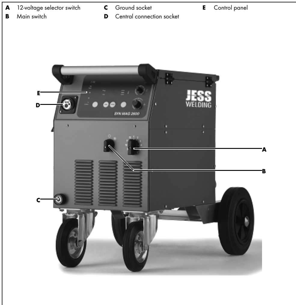
Fig. 9 SynMag 2600/3100 functional description
